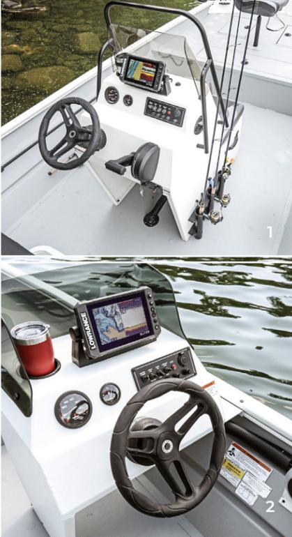
1. Command console with optional side mounted rod holder (CC shown)
