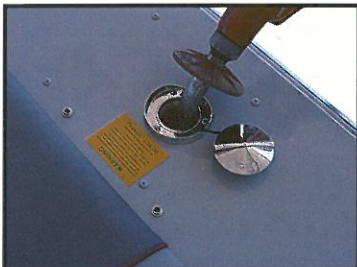
Built-in gas tank
