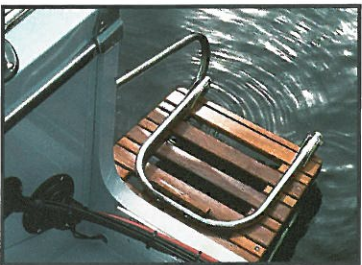
Boarding platform (Baron, Tyees)
